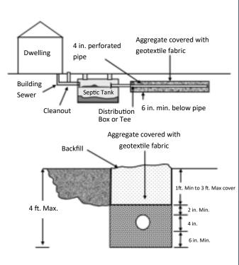
**Cross Section of a Gravel System**
