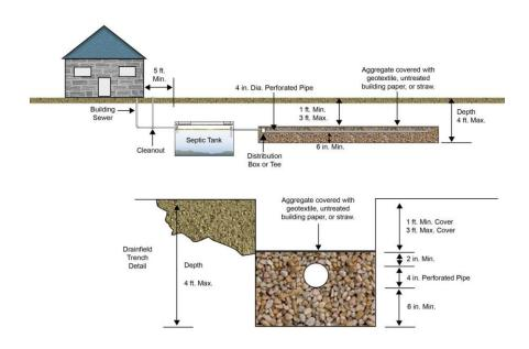
A standard system consists of a septic tank, and a rock-and-pipe drainfield trench.
